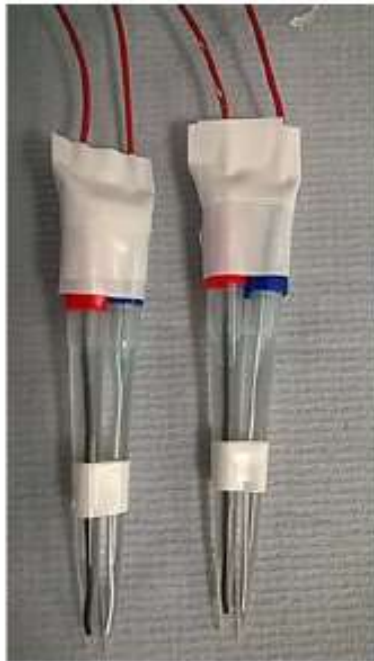
Nitrate selective / reference membrane casting
